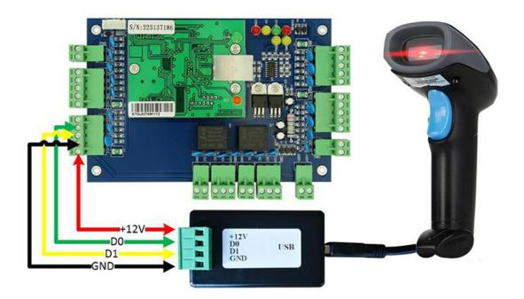
USB-WG converter Connect it to 12V and GND on ACB board, USB scanner connect to USB directly...
